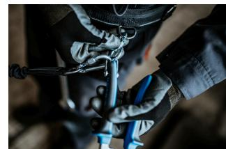
Open the carabiner on the belt and remove the tool, which is attached to a lanyard, from the carabiner on the belt. The tool is now ready for use.
