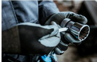
Using the socket remover (Article 1111) depress the pin in the hole while removing the socket from the square drive of the ratchet and then switch the socket or extension.
