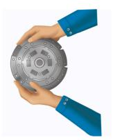
Manually centre the disc on the spring plate.
