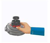
Tighten knob (3) until it touches the spring plate but without blocking the knob.
