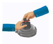
Keeping the knob (2) in place, turn knob (1) and block the expanding cone in the centre of the clutch disc.
