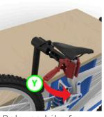
Release bike from stand? To release, firmly hold bike frame. Flip handle (Y) to quickly release tube from the jaw.
