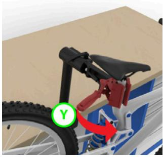
Release bike from stand? To release, firmly hold bike frame. Flip handle (Y) to quickly release tube from the jaw.
