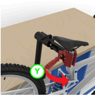
Release bike from stand? To release, firmly hold bike frame. Flip handle (Y) to quickly release tube from the jaw.
