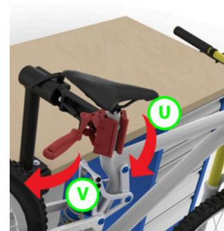
Adjust opened jaw (U) to seatpost or bike tube. Turn handle (V) until jaw firmly grabs the tube.
