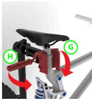
Adjust opened jaw (G) to the seatpost or bike tube. Turn handle (H) until jaw firmly grabs the tube.
