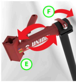
Adjust jaw angle and clamp bike safely? To adjust the bike stand jaw angle, release lever (F) and adjust/rotate (E).
