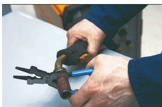
Nozzle removal and installation
