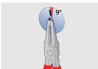
The tips are inserted into the jaw at an angle that prevents the circlip from sliding off the tips
